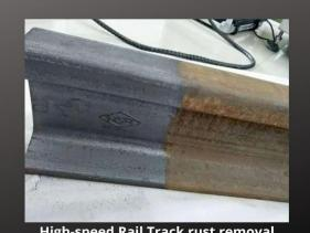
High-speed Rail Track rust removal
